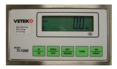
All Scales are EC type-approved non-automatic weighing instrument Accuracy class III Basically, the Weighing Indicator (TI-1200-S), is the same in all Scales.
