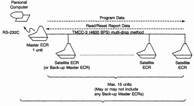
Max. 16 units altogether in one system loop.
